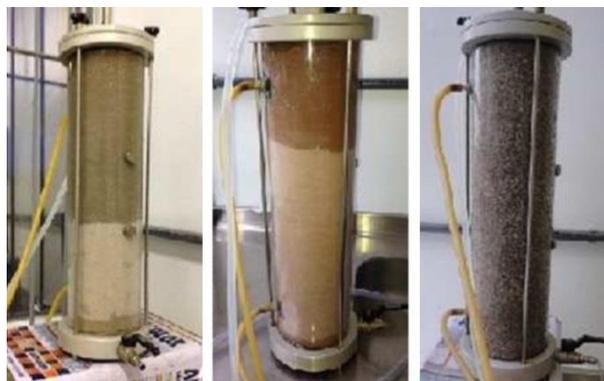
FIGURA 11 – PERMEÔMETROS UTILIZADOS NOS ENSAIOS
