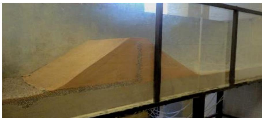
FIGURA 21 – MODELO FÍSICO DA BARRAGEM
